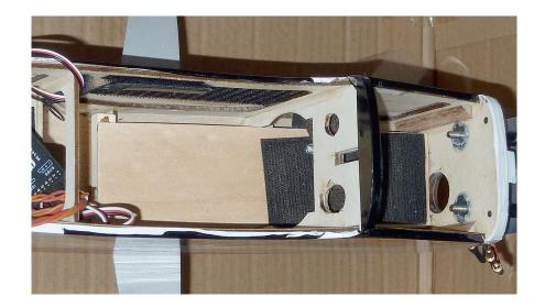
**6 Film.** Before cutting the film out of the fuselage air outlet, wing servo holes, wing wire holes and elevator and rudder control exits, I went round the edges with a film iron. The film was not strongly glued down on the sheet and might pull away with time. I was a bit concerned that a single warm air outlet would not be enough. When I fitted the cowl I saw that air from the motor could also come out through the side gaps.
